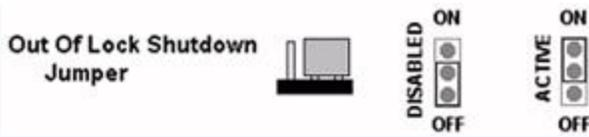
The 1W PLL features out of lock shutdown, this is always required for legal use when the transmitter is connected to a radiating antenna. The diagram above shows how to set the jumper to activate it.
