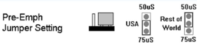
If the 1 watt PLL is connected to a Veronica / Aareff Limiter Compressor or a Stereo Coder, pre-emphasis is not required. To disable the pre-emphasis, do not select 50uS or 75uS and remove the jumper completely. Store the jumper in a safe place just in case you need to restore the pre-emph for another application at a later date.
